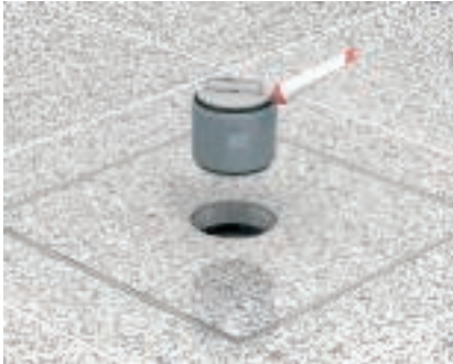
Cleaning of the seals To complete the mounting work, clean the interior of the cassette and the seals of the cassette and tube body. Apply Vaseline to the seals (contained in the scope of delivery).
