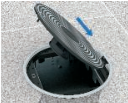
Installation of the hinged cover Attach the lid with an opening angle of 45° in front of the hinge seat and push it back.
