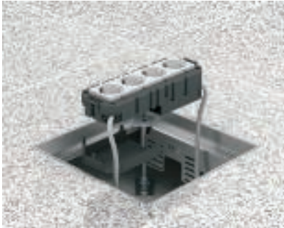
Device mounting in MT module support Devices are mounted in the module support MT3/45 and MT4/45 outside the cassette. After cable connection, insert the module support into the cassette frame from above.
