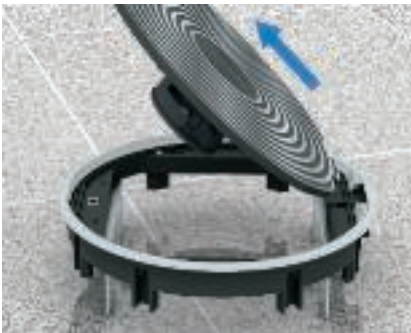
Expansion of the hinged cover Raise the lid by approx. 45° and pull it forward on one side.
