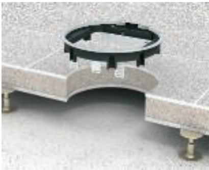
Mounting of GRAF9 in raised and cavity floor When used in raised and cavity floors, the universal fixing bracket acts as an expansion claw. Tighten the screw with max. 4 rotations. The claws fasten the service outlet in the mounting opening.
