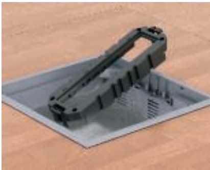
Installation of the module support in a service outlet or a cassette Insert the module support in the locking ladder of the service outlet or the cassette and lock it in the locking ladders on both sides.
