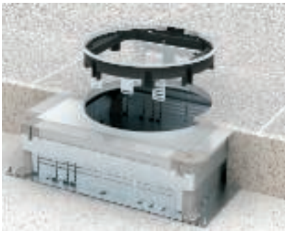
Mounting of GRAF9 in duct systems Insert the service outlet into the blanking lid from above and screw it tight. The fixing unit grips under the blanking lid.
