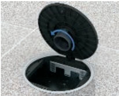
Unlocking of the tube body Open the lid, unlock the tube body by turning it to the left and push it up.
