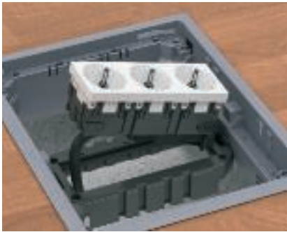
Installation of a triple in the module support Lock the connected socket unit into the module support from above.
