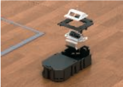
Device mounting in GB mounting boxes The device is mounted without screws in cover plates and GB mounting boxes. Note: Lock Modul 45 devices into the cover plate for connecting the cable.
